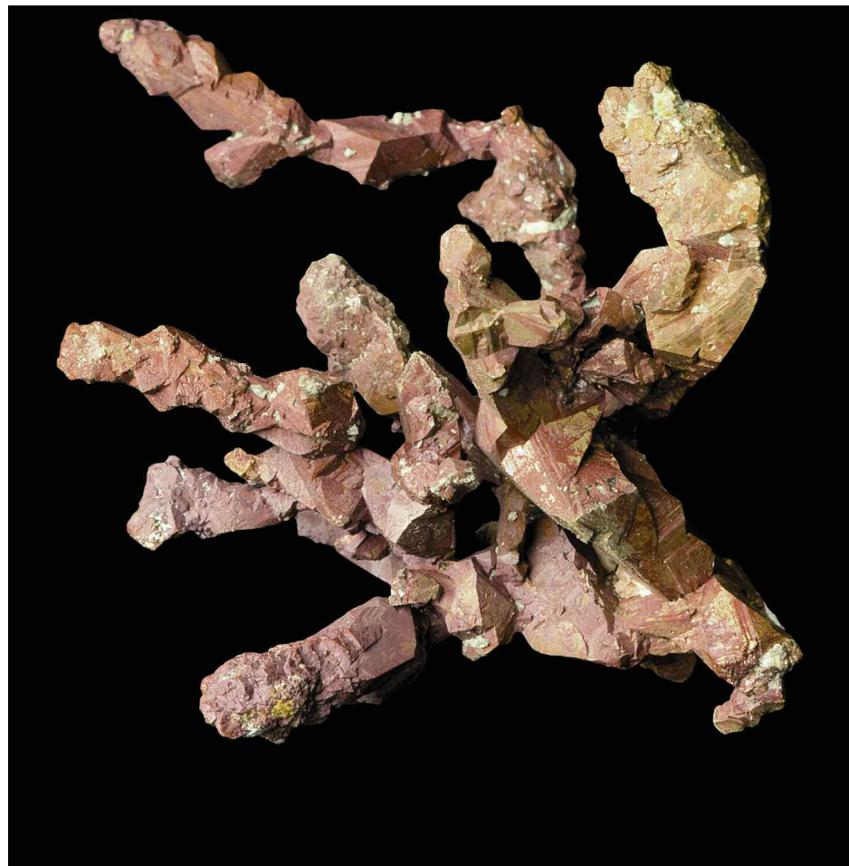
Fig. 7. Dendrite of native copper coated by cuprite film, 6 cm. Specimen: Russian Minerals Company . Photo: Stanislav I. Pekov.
