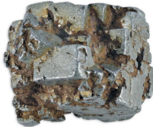
6.60. Multi-terminated cubic crystal of placer-forming platinum minerals with rough blocky-mosaic surface, rare morphological type. Width 1.80 cm, density 14.03 g/cm<sup>3</sup>.
