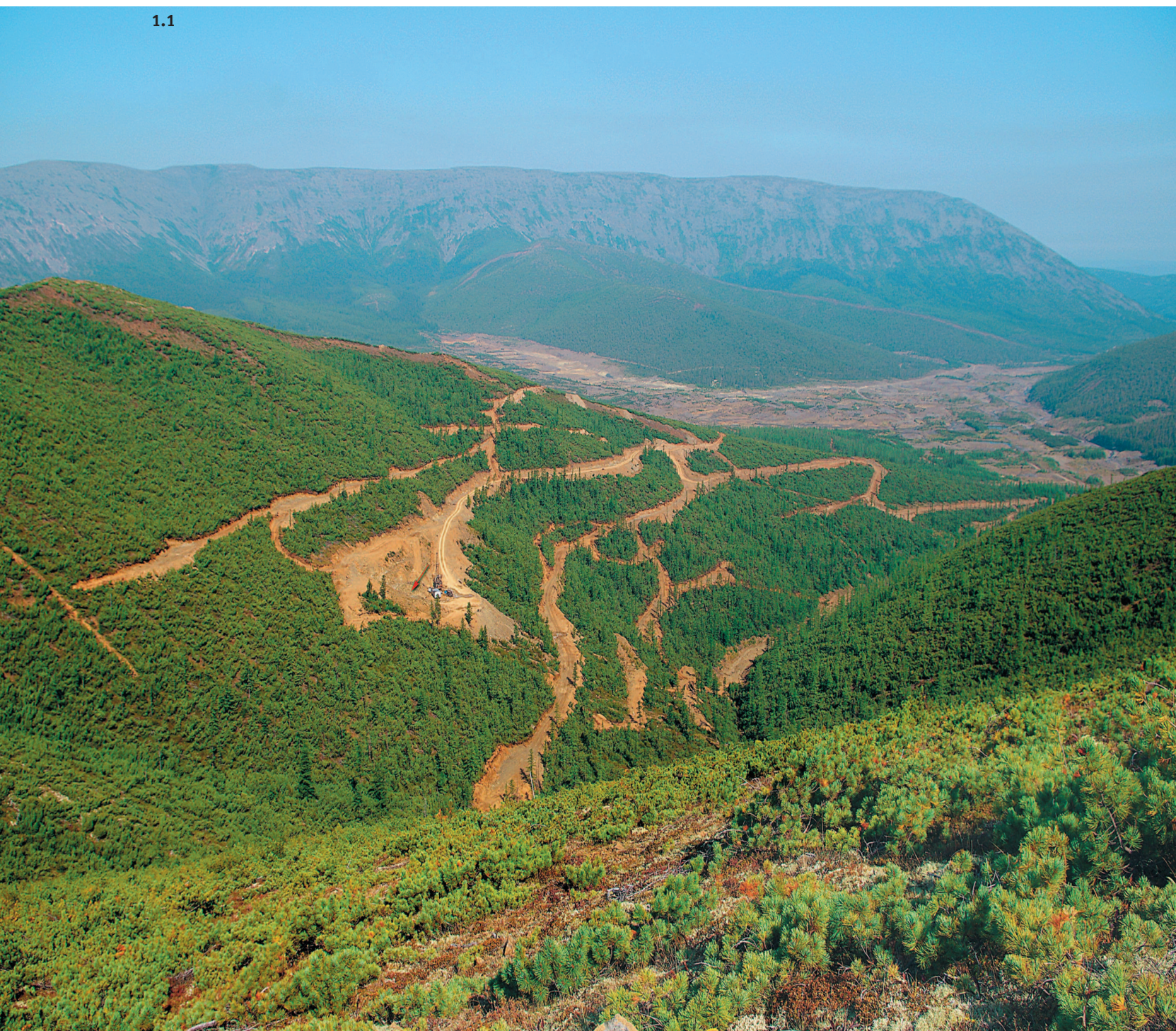
1.1. Left slope of the Maly Creek valley is composed of dunite with the platinum-group minerals occurrences in chromitites. Exploration trenches and drill lines are along the roads. Open pit of the Verkhnee platinum-group minerals prospect (indicated by arrow). At far is the northwestern part of the Konder ring range, at the bottom of which boulder-sand-pebble mixed technogenic sediments of abandoned placer of the Konder River upstream and flowing creeks are present. Photo of 2011.
